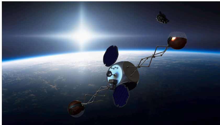
Fig. 14. Sling-Sat method: a tri-scissor arm approach [126].
