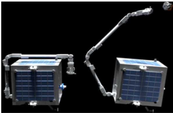
Fig. 6. Space robotic arm attached to a spacecraft, both stowed and partially deployed [83].
