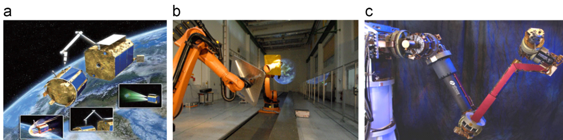
Fig. 3. Single arm capturing methods: (a) DEOS [23]. (b) EPOS [25]. (c) FREND [27].
